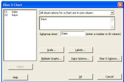
**8** Click **Xbar-S Options**, then click the **Tests** tab. Notice this dialog box reflects the tests and test values you specified earlier. (See *Set options for control charts* on page 4-2.)
