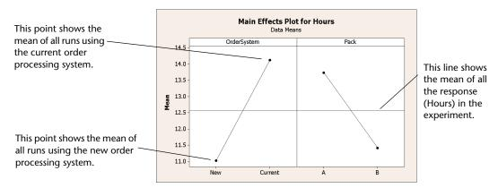
The order processing system and packing procedure have a similar effect on order preparation time. That is, the line connecting the mean responses for the new and current order processing system has a slope similar to slope of the line connecting the mean response for packing procedure A and packing procedure B. The plot also indicates that orders using:
