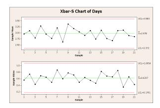
The  $\overline{X}$  and S chart now includes the new subgroup. The mean ( $\overline{X}$  = 2.978) and standard deviation ( $\overline{S}$  = 0.6207) have changed slightly, but the process still appears to be in control.
