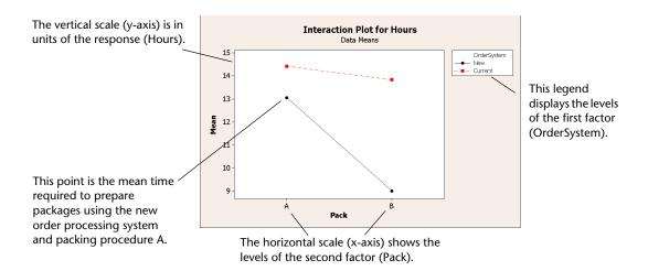
An interaction plot shows the impact that changing the settings of one factor has on another factor. Because an interaction can magnify or diminish main effects, evaluating interactions is extremely important.
